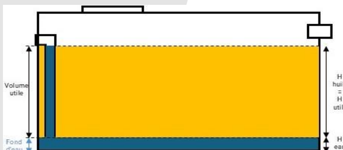
Figure 4 : Emergency operation : complete leak of 100% of the oil volume, retained in the DEPOSIT®
