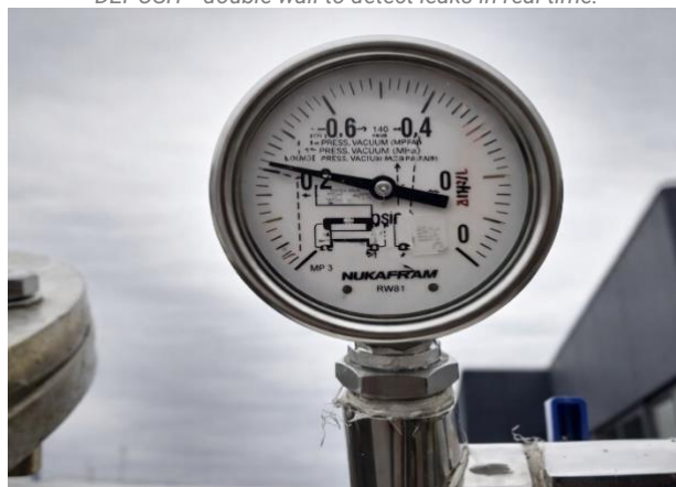
Control vacuum gauge allowing measurement and monitoring of the pit's watertightness.
