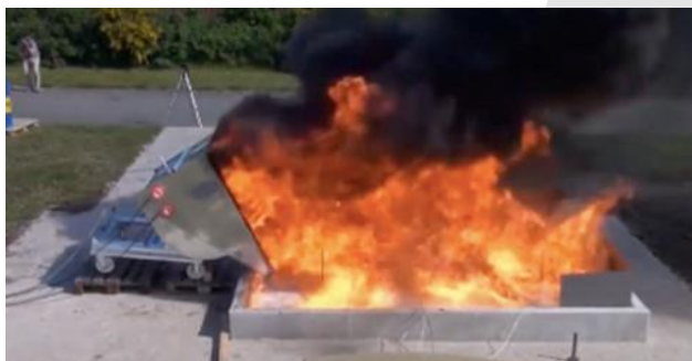
Example of laboratory testing of an EXTICOV-LHD® fire-protection cover on a recovery pit.
