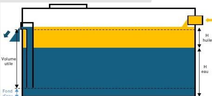
Figure 3 : Incident operation in the event of a minor transformer leak
